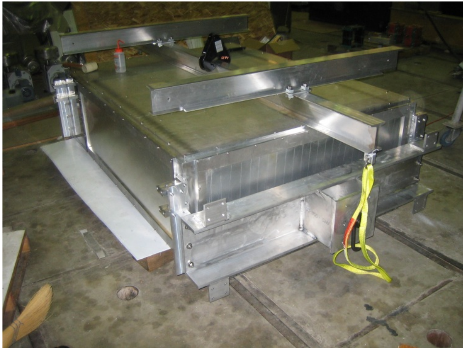
FIG. 1. Photograph of the SAMURAI TPC enclosure with motion chassis attached.
